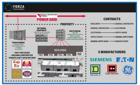
As more power is pushed into or out of the grid, bigger equipment is required, which increases the underlying lead time.
